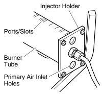
Figure 29 - Injector Holder On Outlet Burner Tube
